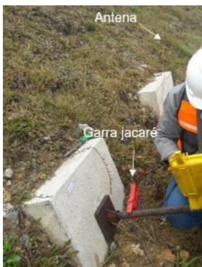
Figura 111 – Ensaio Reflectometric Impulse Measurement Technique
